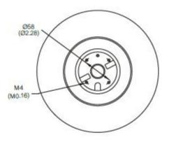
\* Caution: Assembly screw mounted in the MOTOR length is not more than 5mm
